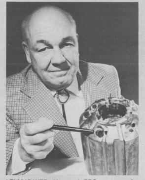
LENNY BAKER with an early PDC pressure-coring bit that he designed while at Sandia.
